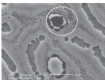
Fig. 6. SEM image at higher magnification (5000x) of sample from the metallic crown; in detail A is a different shape particle
